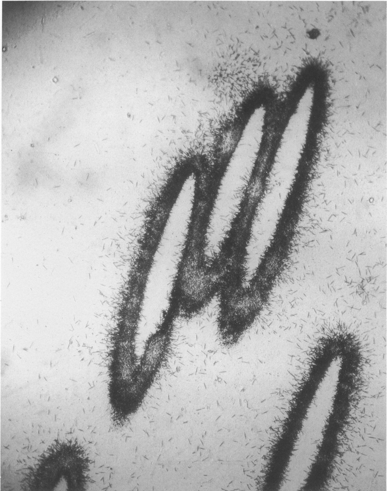
Figure 5 Uranium distribution in taper-sectioned Nb-Nb 3 Sn-Sn wires. Uranium is confined to the two outer layers, Sn and Nb 3 Sn.
